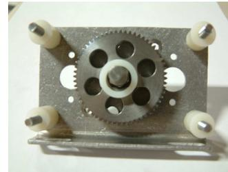
Step 4: Place the second Motor Plate onto of the assembly. Make sure that the curve is on the opposite side of the screws.
