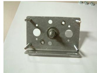
Step 2: Put the 60T 32dp Gear onto Output Shaft.
